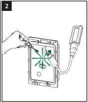
Max) until the fixed GREEN LED lights up. On the key, the RED LED will light up Release the button, and check for GREEN flashing and at the end the escutcheon flashing.
