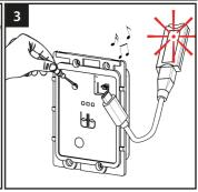
Connect the master key to the Press the programming button (0 ÷ Press the programming button again. escutcheon. Start the ULIXE app on 3 sec. Max) until the steady RED LED On the key, the RED LED will light up your smartphone, access the reserved lights up. Release the button, and flashing and at the end the knob will area and follow the procedure. check the flashing RED.
