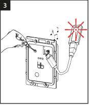
Press the programming button ( $3 \div 6$  sec. Press the programming button again. will sound an increasing tone.
