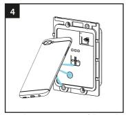
the smartphone, follow authentication procedures, bringing it close to the brightness sensor which will receive flashes of light emitted by the smartphone. Once finished the device will be paired.
